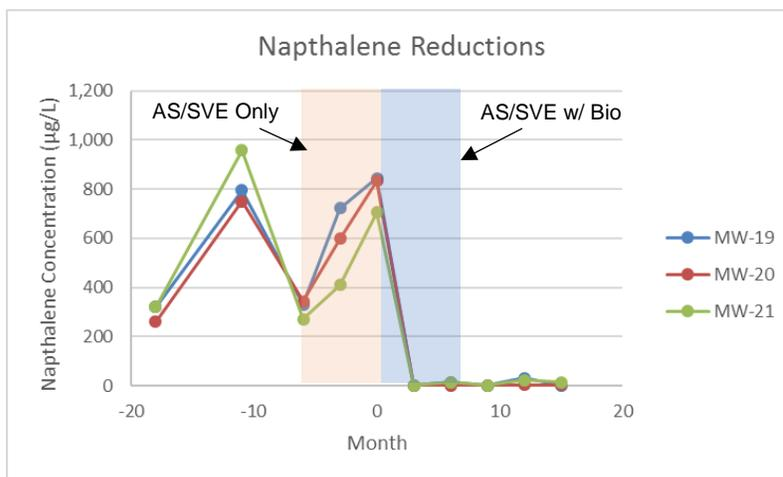
**Reductions achieved by the AS/SVE system operation had been unnoticeable prior to biological enhancement. Incorporating biological enhancements and nutrients with the AS/SVE system created the ideal aerobic environment for bioremediation.**
