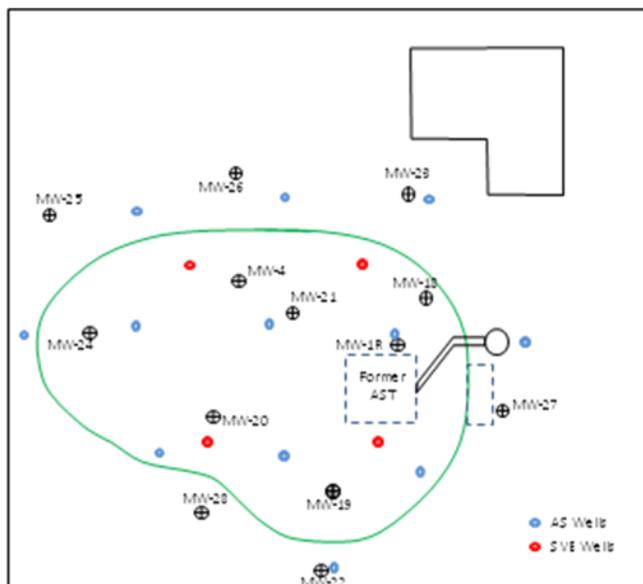
The AS/SVE system was designed to operate for a total of twelve months. After six months of treatment, the decision to enhance the performance of the system with biological enhancements was made. ETEC was contracted to provide biological enhancements and nutrients for the remaining five months of active treatment.
